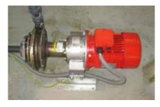
Feeding itself takes place via a speed-controlled two-stage centrifugal pump. This is insensitive to dry running and foreign objects and, despite its high pump performance, is characterized by particularly low wear.
